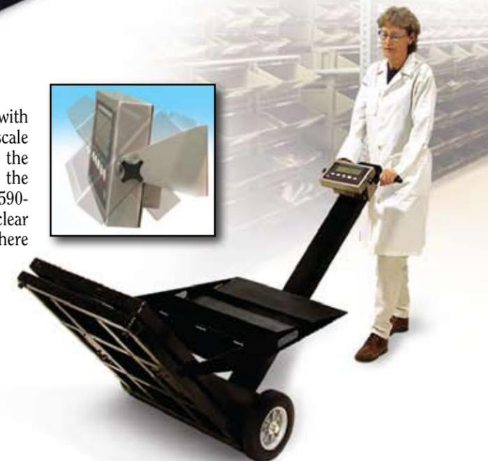
The portability frame and caster engaging mechanism are below the scale's live rails for unconfined weighing of pallets and other large items.
