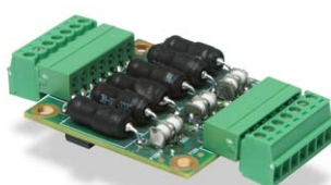
Severe Transient Voltage Suppressor (STVS) Added protection against voltage surges such as those caused by extreme lightning.
