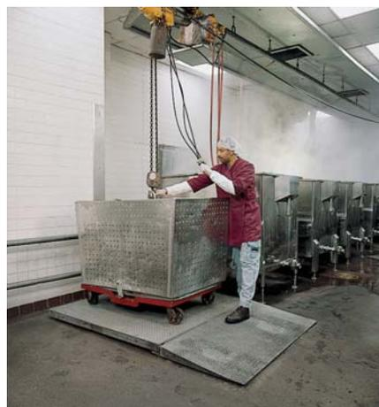
The ProDec's solid deck construction maintains a high resistance to damage from overload and shock. Stainless steel deck construction protects from corrosion in harsh environments.
