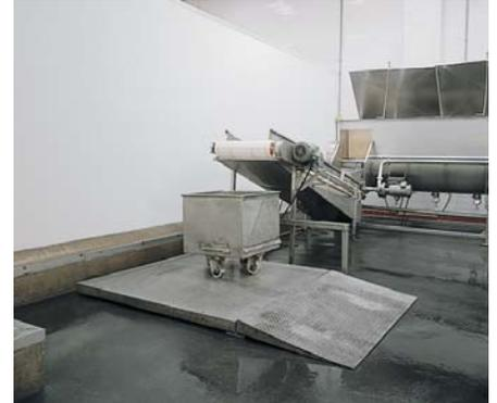
Correct positioning of the ProDec speeds up work flow. Place ramps on one, two, three, or four sides to create optimum traffic patterns.
